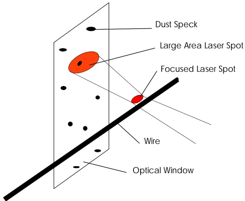
Fig. 3: The optical concept of ALS12XY and ALS13XY laser gauges.
