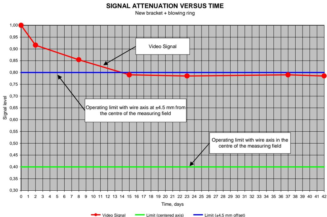
**Fig. 8: The diagram shows the plot of the video signal level versus the operating time. No cleaning was needed during the test. The new "self-cleaning" protection has been used.**
