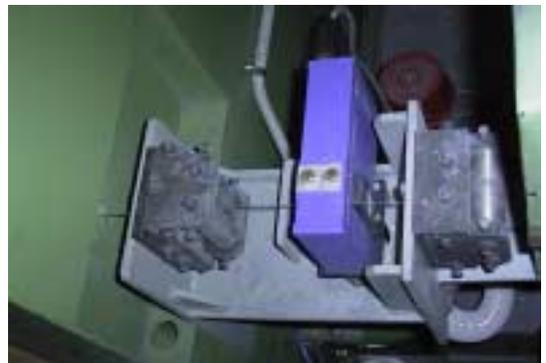
**Fig. 6: Application of ALS13XY laser gauge on a dry drawing bench.**
